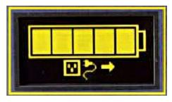
Levelling of the elements should always be done after charging the batteries. Watering a battery before charge (or with a low charge level) can lead to boil-over, resulting in potential bodily injury and potential damage to the watering system and the battery.
