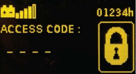
• Validation by pressing on is active only if access code is known and entered - refer to maintenance manual for the procedure for the different level code useage
