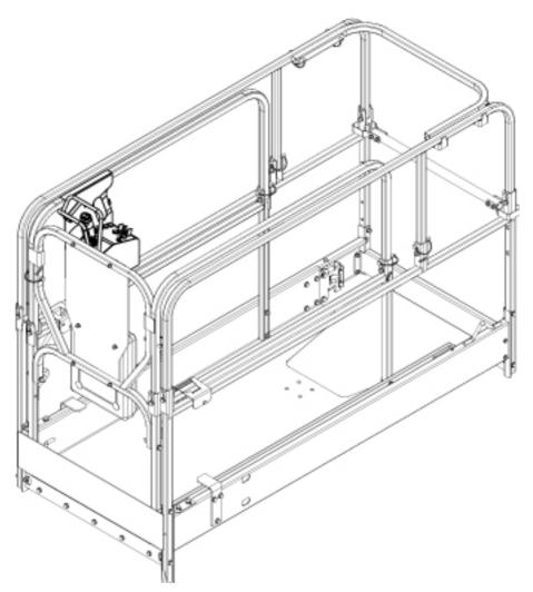
Remove platform control box from its designated position and place it on platform floor
