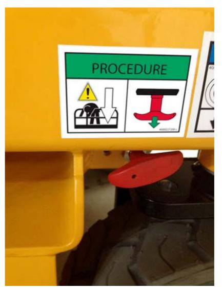
**N.B.-:-P**ULLING ON TO THE **T**-HANDLE, IMMEDIATELY ACTIVATES THE EMERGENCY LOWERING OF THE PLATFORM.
