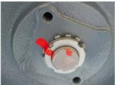
• Straighten the bent tooth of the washer which restricts the nut rotation. Use a screwdriver and a hammer.
